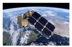
Sentinel-2 satellite for wide-swath, highresolution multispectral imaging
